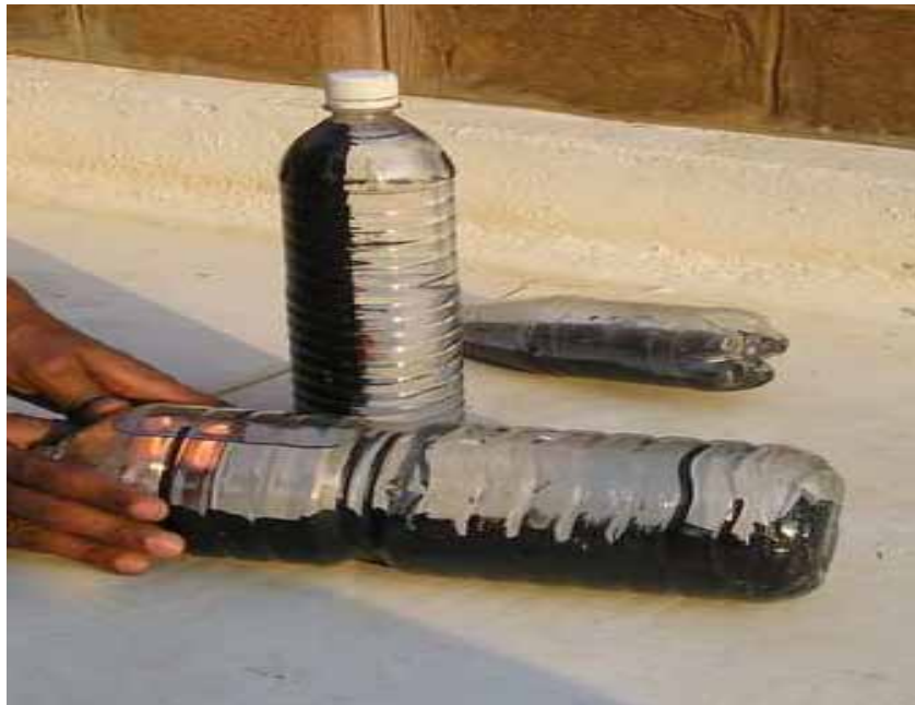
Solar disinfection or SODIS using a bottle painted half black
